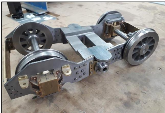
As many will know, the King bogie has the leading wheels on the inside of the frames and the trailing wheels on the outside of the frames. Accordingly,
