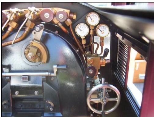
who was building the same locomotive in 7 ¼." This locomotive was a traditional mallet with the four cylinders compounded in two pairs. The 3'6" gauge prototype was built in 1920's in Holland. The attention to detail on the model was stunning with fully working scale controls, including vacuum brake. This was complimented by a working tender water gauge (pointer around a semi-circle), re-railing jacks and
